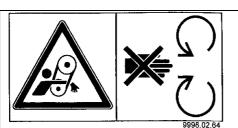
Never open or remove any safety guards when the unit is running.
