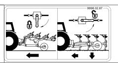
Before transporting on roads, set to lock position with the shut-off valve open.
