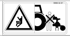
Risk of crushing in and around the tractor and the implement! When coupling the implement combination to the tractor, ensure that no one is standing within the operating areas of the tractor or implement! Do not step between the tractor and implement to operate the external three-point hydraulic controls.
