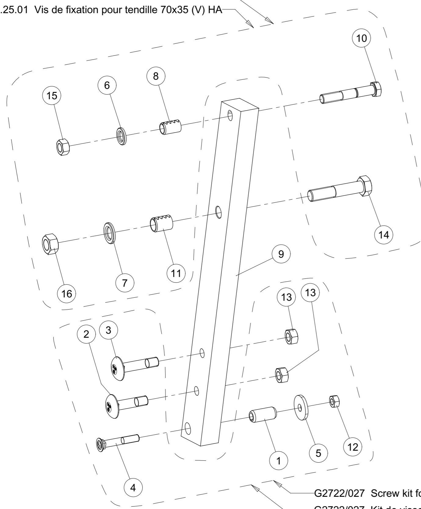
G2722/027 Screw kit for the Leg (thickness 35)
