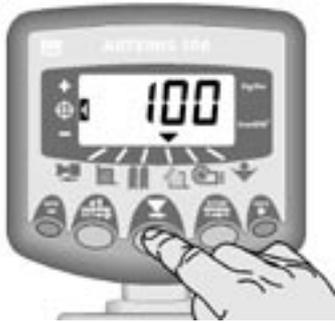
Figure 11 View Drilling Rate (kg/ha)
