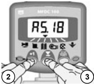
Figure 29: Set Tramline Bout for 10-bout/18-bout tramlining
