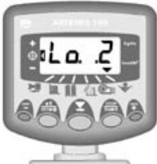
Figure 31: Hopper 2 Low Alarm
