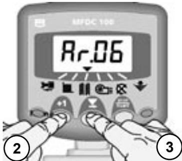
Figure 28: Set Tramline Bout for Assymetrical Right tramlining
