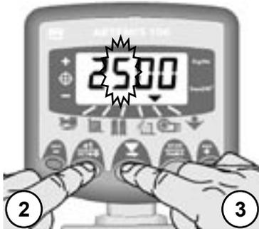
Figure 22: Change Fan Alarm Speed
