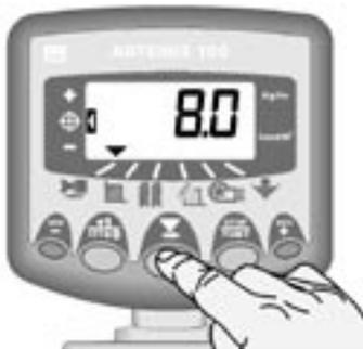
Figure 1 : Select Fwd. Speed channel
