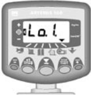
Figure 30: Hopper 1 Low Alarm
