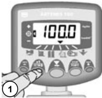
Figure 12 View current Target Rate
