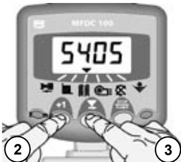
Figure 26: Set Tramline Bout for Symmetrical tramlining
